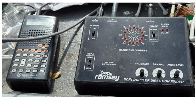
Figure 6. Doppler radio direction finder connected to a VHF/UHF scanner tuned to the tag frequency; the LED ring shows the bearing.
