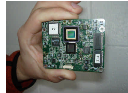
FISM-1CS Module with Dual Image Sensors
