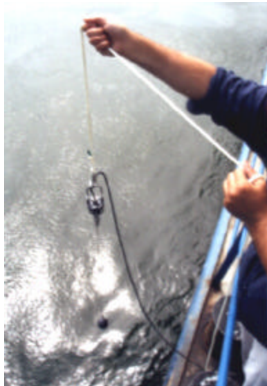
Figure 2: A Sonar Transducer is lowered over the side of the Surface Vessel
